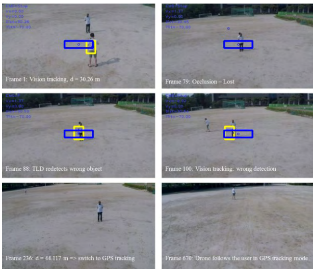
Fig. 10. Visual – GPS switching caused by wrong detection: 1) Start tracking at Vision tracking mode. 2) The user appearance is occluded by a similar object. 3) The object tracking algorithm then detect the similar one (miss-detect the target object) 4) The target object keeps moving. At a moment, the distance between the drone and the target object is more than the initial distance + threshold (10 meters), our algorithm switches to GPS tracking mode 5) The drone follows user in GPS tracking mode 6) If the drone can redetect the user => switch to Vision tracking mode
