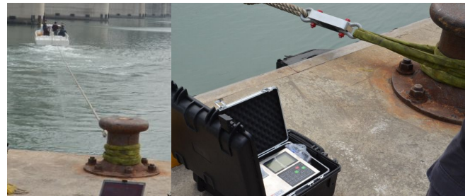
Fig. 1. Sea trial for towing force of two types of netboats.
