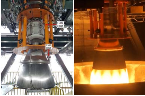
Fig. 2 Combustion chamber & Firing test
