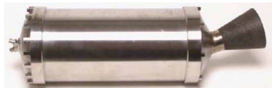
Fig. 1 STAR 8 served as the RAD motor on the Mars Exploration Rover program of the Jet Propulsion Laboratory
