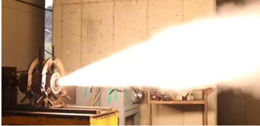
Fig. 4 Ground Combustion Test of KSLV-II Ullage Motor
