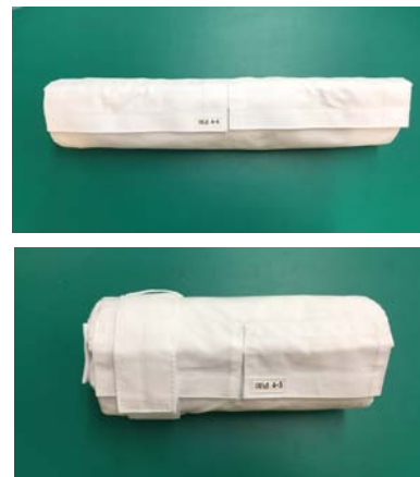
Fig. 3 Cryogenic Insulation for Recirculation Line
