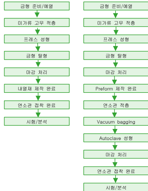
Fig. 1 Process of Insulator Manufacturing (left : Hot Press Molding, right : Unvulcanized Insulator Method)
