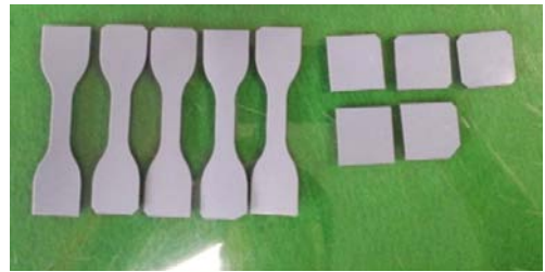
Fig. 3 Specimen for Accelerated Lifetime Test, Left (tensile strength, elongation), right (volume / weight / thickness)
