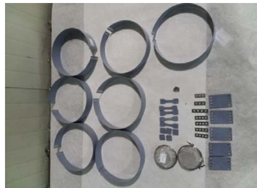
Fig. 8 Disassembled Fluororubber Composite
