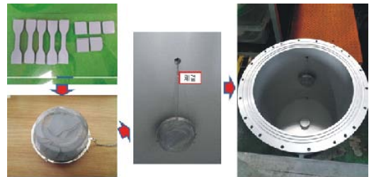
Fig. 4 Tightening Sequence of Specimen And Storage Container for Lifetime Test
