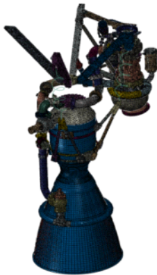
Fig. 1 Finite Element Model for 75 tonf-class engine
