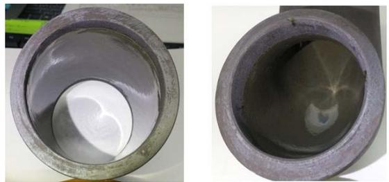
Fig. 12 Coated specimen (straight pipe, elbow)
