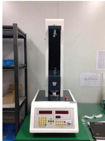
Fig. 7 Experiment instrument for spring force
