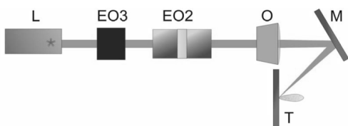
Fig. 3 Concept of the electro optic steering system[10].
