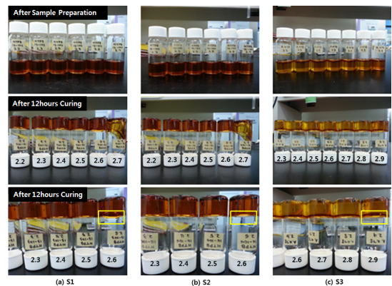
Fig. 1 Result of Functionality of HTPBs (a) S1 F : 2.5 (b) S2 F : 2.5 (c) S3 F : 2.8.
