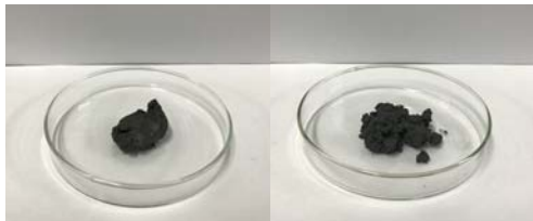
Fig. 3 Kerosene gel wrt metal particles addition (left: 10 wt%, right: 20 wt%).
