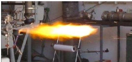
Fig. 1 Hot firing Test using Gel Fuel[4].
