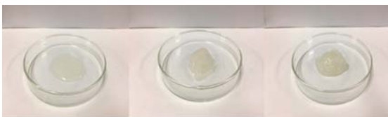
Fig. 3 Nitromethane gel propellant with SS-SIL (left: 5 wt%, middle: 6.5 wt%, right: 8 wt%)
