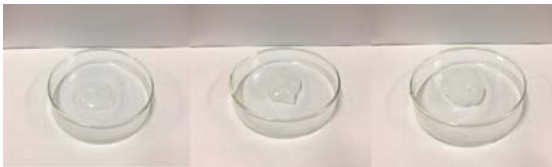
Fig. 2 Nitromethane gel propellant with Aerosil (left: 5 wt%, middle: 6.5 wt%, right: 8 wt%)
