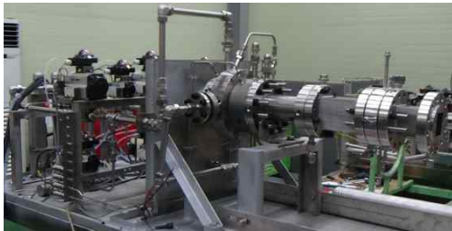
Fig. 2 Photo of Test Stand for Vitiated Air Heater
