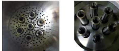
Fig. 6 Photo of injectors after tests
