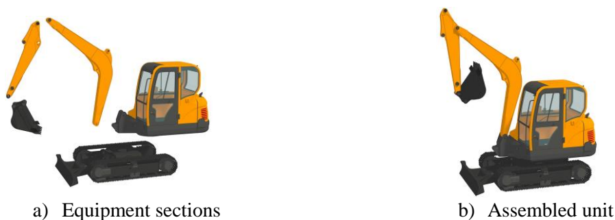
Fig. 2. Typical equipment modeling for an excavator
