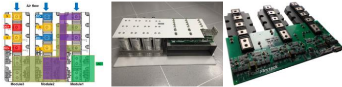
Fig. 4. NPC1 phase arm design: busbar layout, stack and driver board
