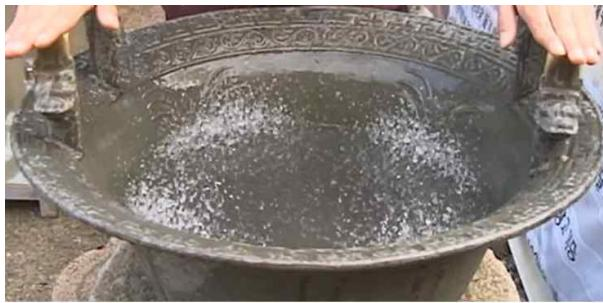
Fig. 1. Resonance experiment using a bronze washbasin
