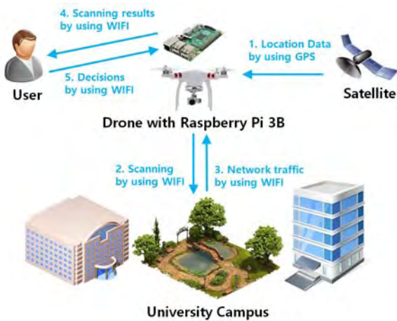
Fig 2 Flowchart for a study of flying intrusion detector using the drone
