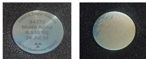
Fig. 1. Alpha-emitting calibration source (SRS 94370).
