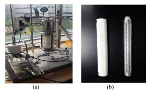
Fig. 1. (a) Candle filtration experiment equipment (b) filter module.
