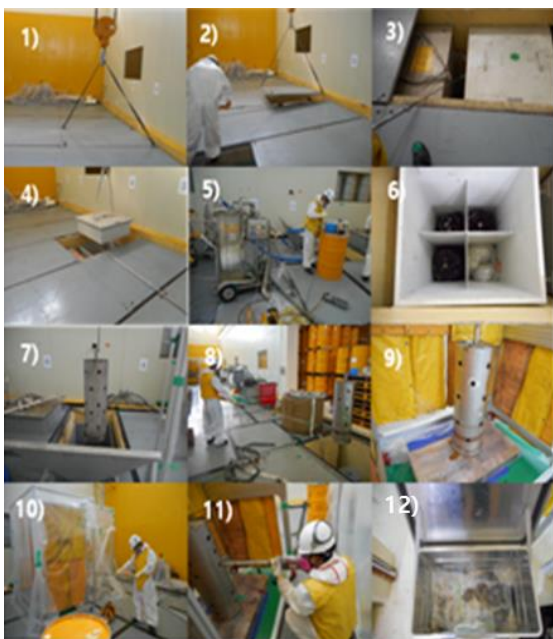
Fig. 3. The procedure for sampling old waste filters.
