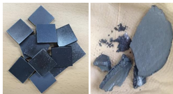
Fig. 1. Carbon steel before melting(left) and slag after melting(right).
