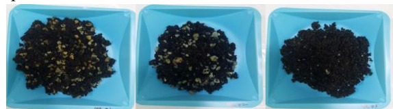
Fig. 2. Spent resin mixture samples from Wolsung NPPs Unit 1.
