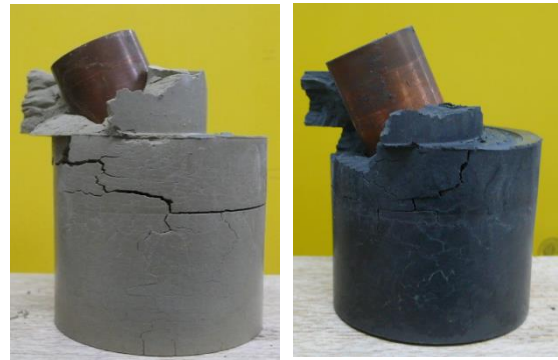
Fig. 3. Shear rotated copper rod in a pure bentonite and a 3 wt% graphite added bentonite.
