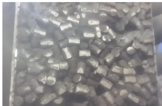
Fig. 1. U metal products in a cathode basket after electrolytic reduction using a carbon anode.
