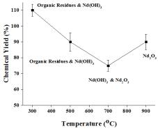
Fig. 3. Recovery rate for Pm-147 with an oxide compound (Nd<sub>2</sub>O<sub>3</sub>) at different temperatures, (a) at 300°C, (b) 500°C, (c) 700°C, (d) 900°C for 1h, respectively.
