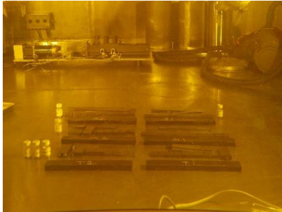
Fig. 5. Dismantled capsule and specimens.
