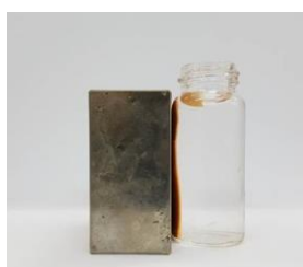
Fig. 2. Magnetically collected clay microspheres after adsorption of Cs.
