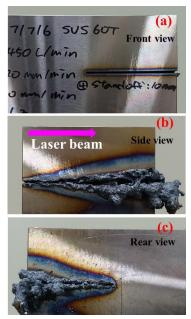
Fig. 2. Stainless steel after cutting (t=60 mm) using supersonic nozzle at 10mm standoff distance. Front face(a), Side face(b), Rear face(c).
