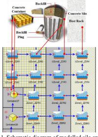
Fig. 1. Schematic diagram of modelled silo and performance assessment module.
