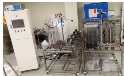
Fig. 2. Semi-Pilot decontamination system(4L/hr).
