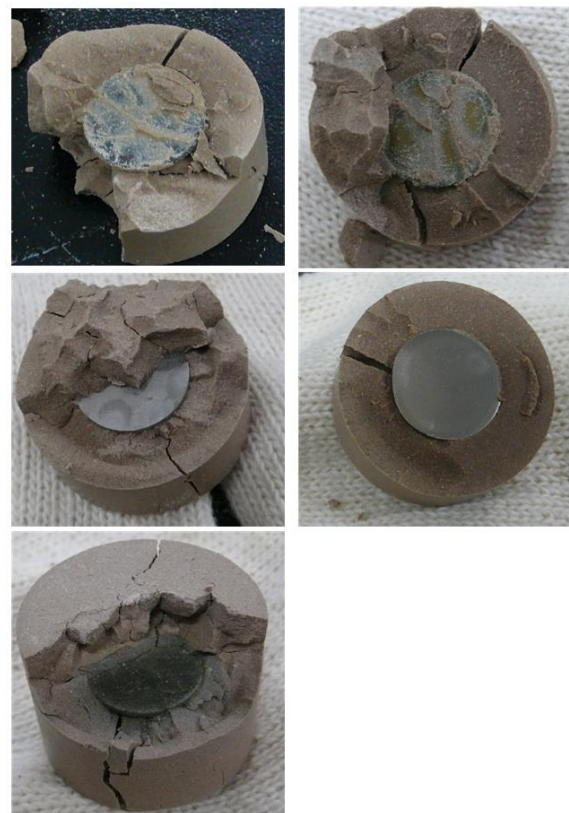
Fig. 2. The 3.2 year old test specimens with compact bentonite right after dismantling.
