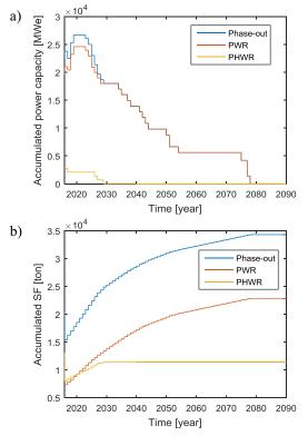
Fig. 1. Accumulated power capacity (a) and the amount of SFs generated (b) in the phase-out scenario.
