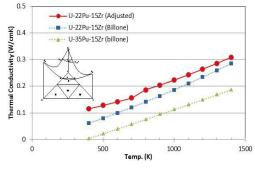
Fig. 2. U-Pu-Zr thermal conductivity comparison.
