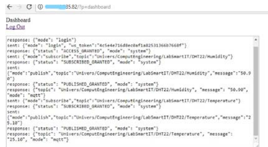
Fig. 4. dashboard of the humidity and temperature data
