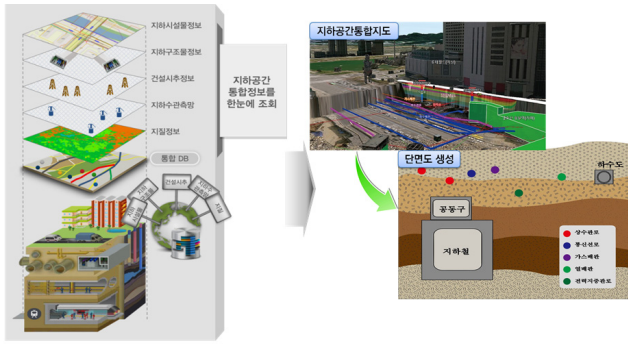
Fig. 1 Concept of underground space integration map
