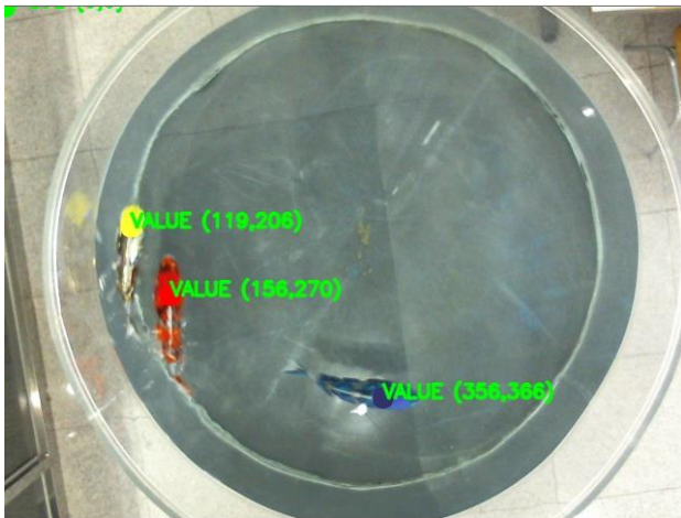
(Figure 6) Position Detection of Fish Robots
