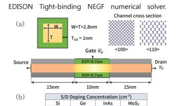
RBT (Reduced basis Transformation) method is used to reduced massive size Hamiltonian, which is calculated from the full-band atomistic tight binding calculation of several hundred to of channel atoms. All calculations set as unstrained NW structure, same as the bulk lattice constant for each material.
