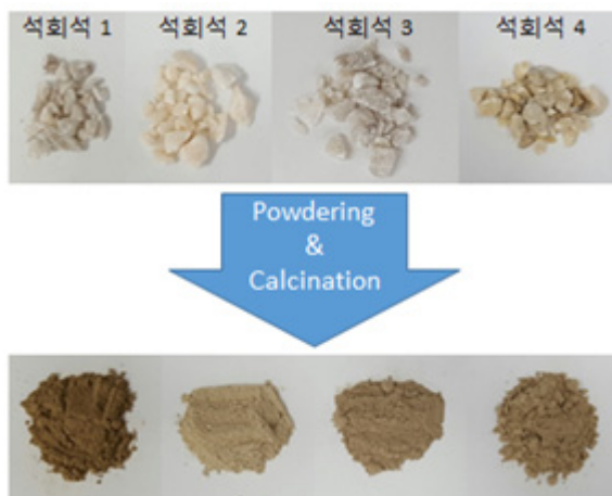
Fig. 1. Forms of the pulverize and calcination process of the minerals.
