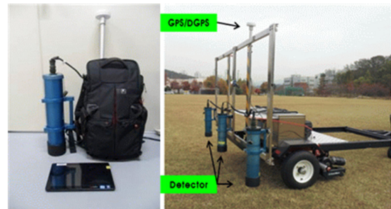
Fig. 1. Site contamination mapping system(backpack and vehicle mount).
