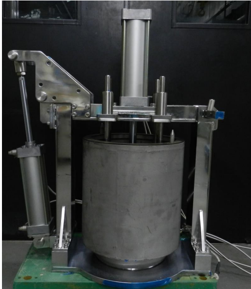
Fig. 1. Press machine for High-Level Radwaste.
