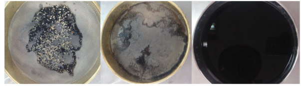
Fig. 4. The image of separation of resin mixture(mesh 850µm/300µm/waste fluid).
