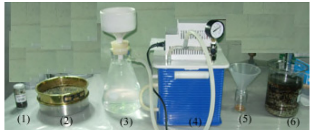
Fig. 2. The image of separation device for resin mixture.
