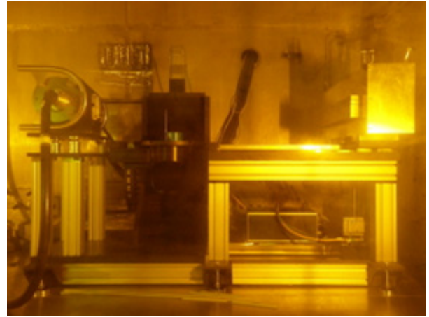
Fig. 1. 450kV X-ray system installed in Hotcell.
