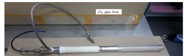
(a) Before assembling (b) After assembling Fig. 2. Anode assembly (type 2).
