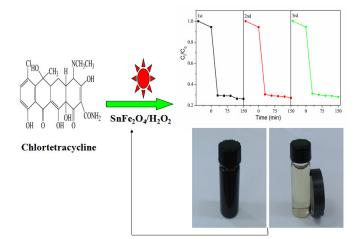
Highly crystalline SnFe<sub>2</sub>O<sub>4</sub> nanoparticles with high saturation magnetization and superior chlortetracycline degradation efficiency was developed using a one-pot solvothermal method.
