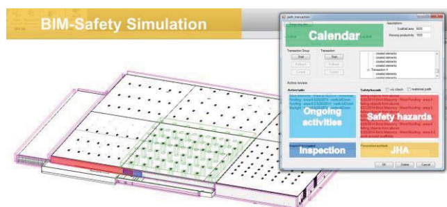
Figure 3. Safety analysis in 4D BIM environment
