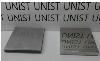
Fig. 1. Surface textures before(left) and after(right) EB treatment.
