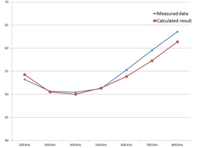
Fig. 2 Transformer temperature according to operation frequency variation
