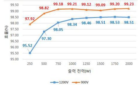
Fig. 6 The comparison between the efficiency of 1200V SiC and 900V SiC
